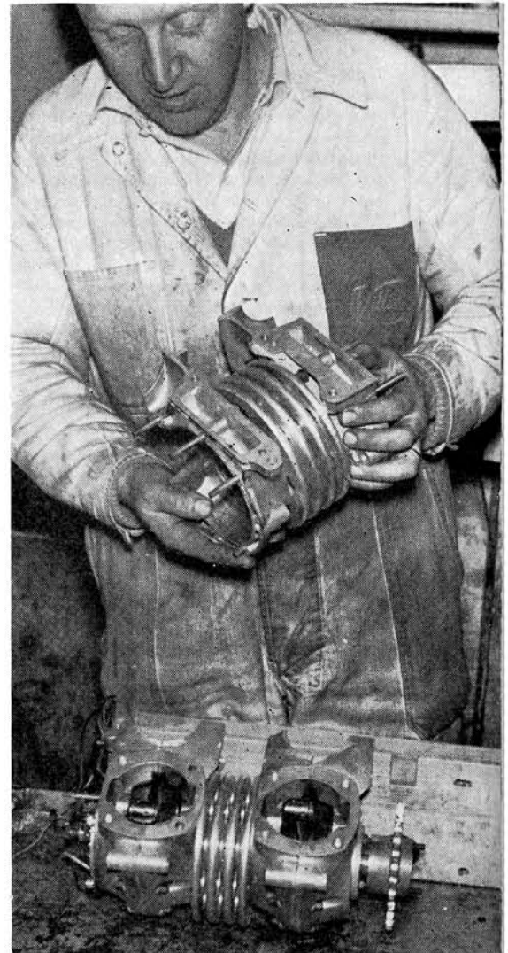
John Dunn is holding one of the crankcase centres from the four-cylinder two-stroke
