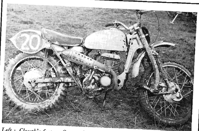
Left: Clough's factory Greeves looks like a standard Challenger but is in fact a 360. Unlike Bickers, Clough still favours the leading-link fork. The latest, spring-controlled, Greeves type has some 6in of movement
